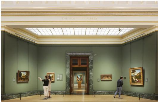
The major feature of the room is its central panelled barrel-vault, flanked by large glazed lay lights to either side. We added soft uplighting from a concealed crosslighting detail to highlight its detail and volume while also softening contrast with the bright planes of the lay lights. Utilising fully dimmable, tuneable white LED sources, the intensity and ambience of the ceiling can be adjusted according to the curators' requirements for exhibitions and events.
